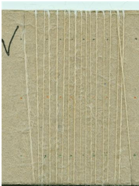
Figure 2: Spinning sample "v" with marked lines for measuring yarn diameter and spinning angle
