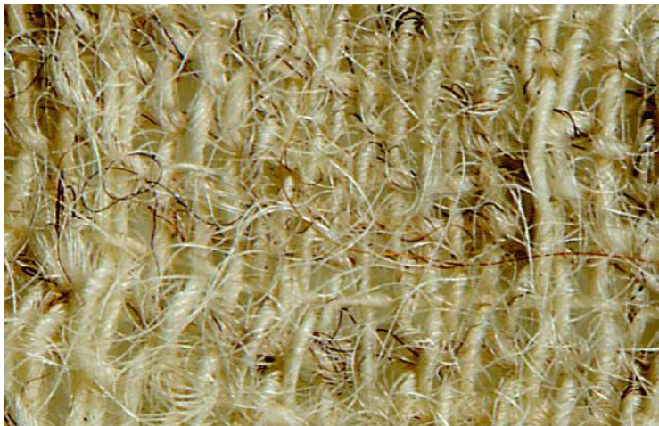
Figure 8: Weaving faults: doubled (left) and floating warp ends (right)
