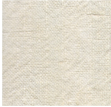
Figure 4d. Balanced tabby, 14 warp and 14 weft threads per cm (linen fabric).
