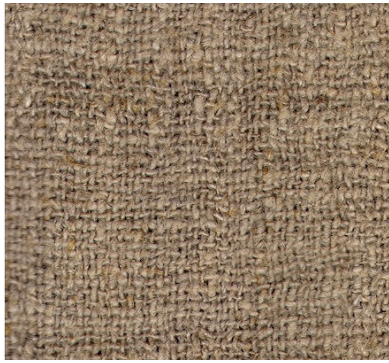
Figure 4c. Balanced tabby, 9 warp and 9 weft threads per cm (wool fabric).
