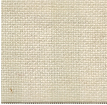
Figure 4c. Balanced tabby, 9 warp and 9 weft threads per cm (wool fabric).
