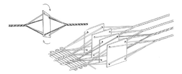
Shematic representation of tablet weaving for the construction of a band. *Drawing: Lise Ræder Knudsen*.
