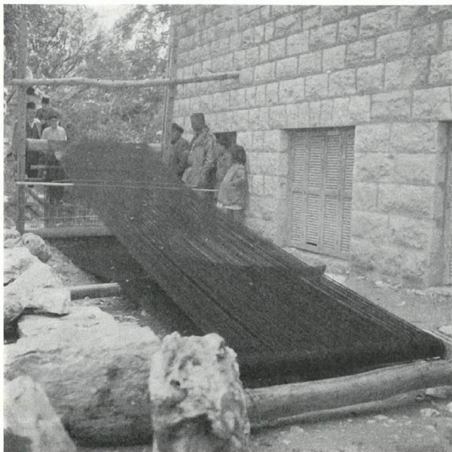
Fig. 40. Tubular loom with three beams built up out of door. Shahime, Lebanon 1961. (M. Hald fot.).
