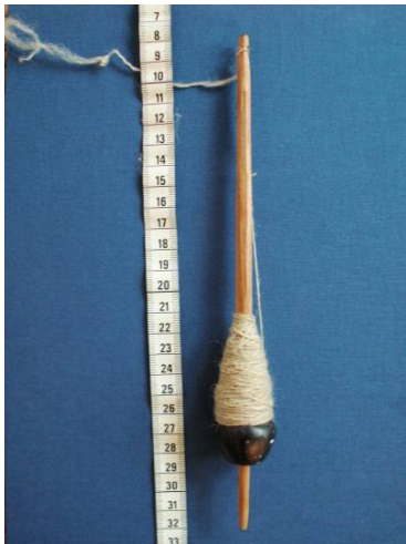
Fig. 8. A filled spindle, 18 g whorl.
