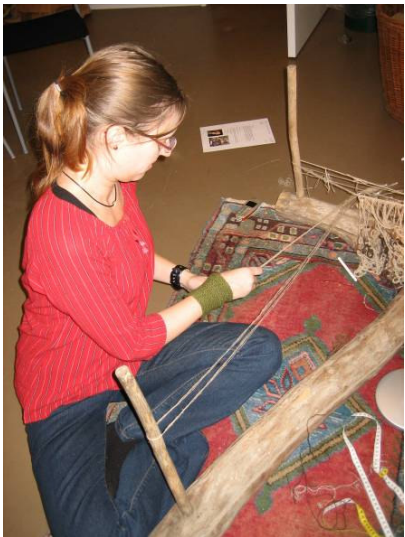
Fig. 19. Warping on a warping frame.
