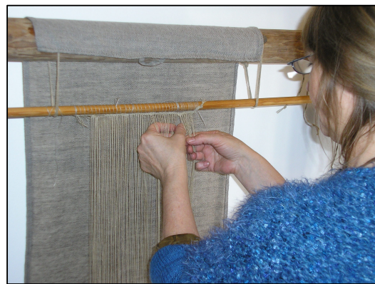
Fig. 14. Arranging the warp threads. The wet handkerchief is seen in the background.
