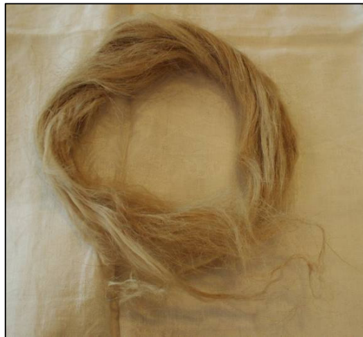
Fig. 1. 10 g of about 50-100 cm long flax fibres used in the experiment.
