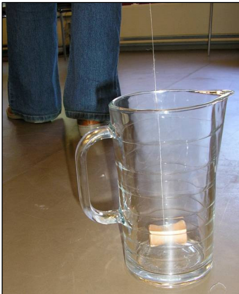
Fig. 8. Ceramic spool with thread on, placed in the glass vessel.
