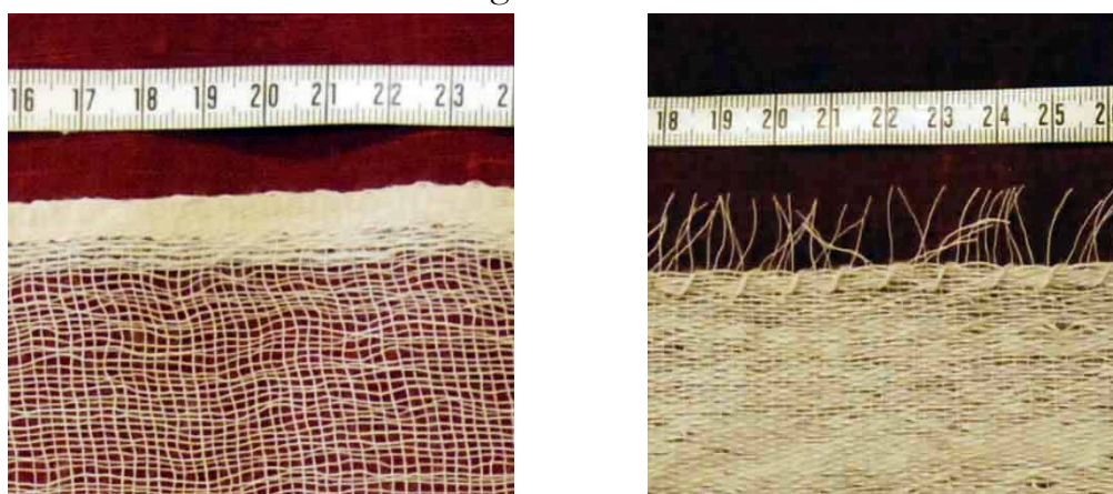
Figure 12. Two fabrics, both woven with threads requiring 10g warp tension. Left: a tabby with app. 5 warp threads per cm and 8 weft threads per cm. Right: a weft faced tabby with app. 6 warp threads per cm and 15 weft threads per cm. (Mårtensson et al. 2007).
